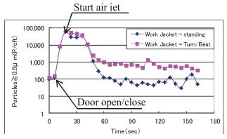
Fig.9 Comparison of particles generated by air jet from work jacket with or without action
