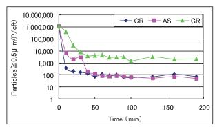
Fig.3 Particle concentration at no operation of Air Shower
