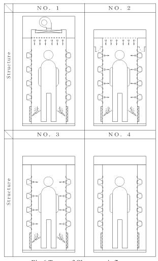
Fig.6 Types of Clean-up air flow
