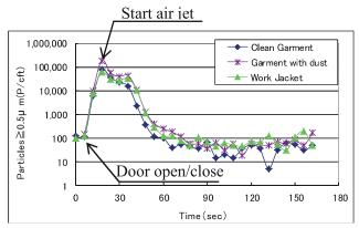
Fig.8 Comparison of particles generated by air jet from garments
