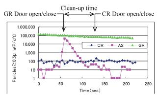
Fig.5 Particle concentration with clean-up cycle
