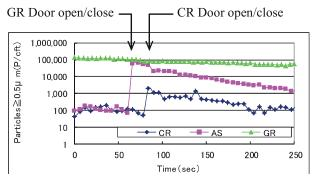
Fig.4 Particle concentration without clean-up cycle
